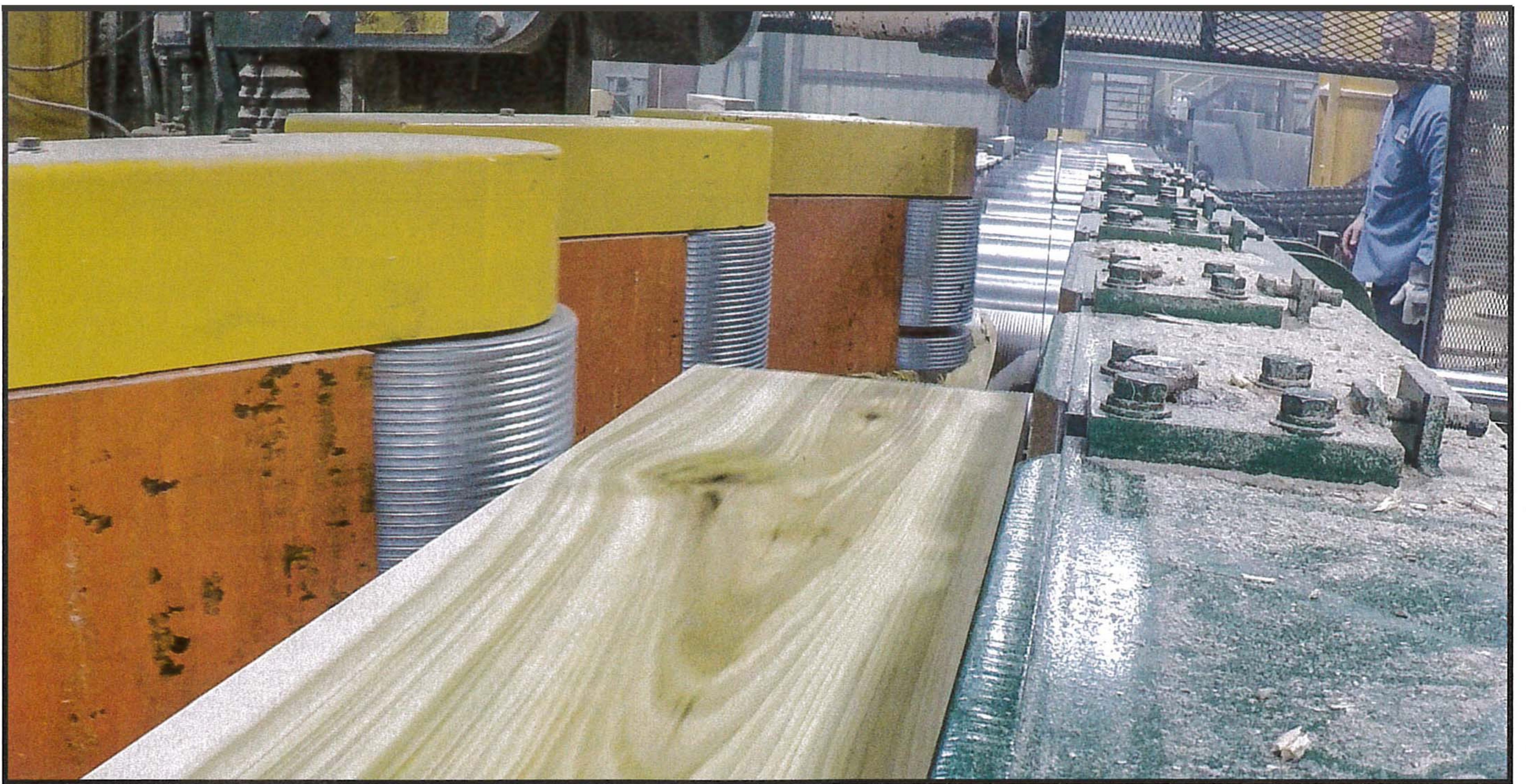
Salem Equipment's new Smart Gate resaw positioner—the yellow and orange elements are press rolls that hold the block against the linebar.
