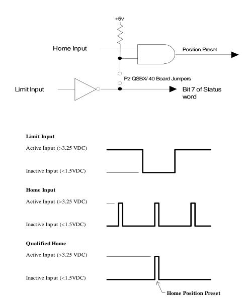
Notice in the figure above (with jumper installed) the Home position is only preset if the Limit is Inactive and Home is Active.
