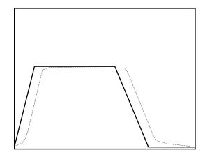
Your valve may have slow response. Add feed forward advance equal to the time between the two speed lines.
