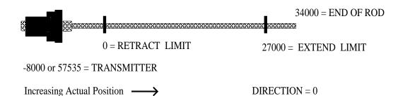
**NOTE:** In this example, positions between the transmitter at -8 inches (57535 in 16-bit math) and the RETRACT LIMIT at 0 inches will cause the axis to move to the RETRACT LIMIT. Positions between 27000 and 57535 will cause the axis to move to the EXTEND LIMIT.
