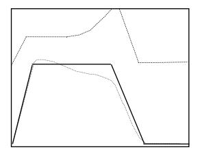
Your pump and/or accumulator may be inadequate (you are running out of oil). Reduce speed, increase pump pressure, add accumulator volume, or get a bigger pump.
