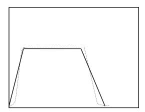
Your valve probably has overlap. Replace the valve with a linear one or try increasing the HYSTERESIS.
