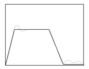
You may have too much hose between the valve and the cylinder. Reduce the amount of hose or add differential gain (usually less than 5).
