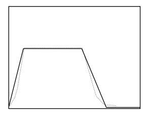
Your valve is probably curvilinear. Replace the valve with a linear one or increase the static gain and tune the system for high-speed stability; expect poor control at low speed and when stopped.
