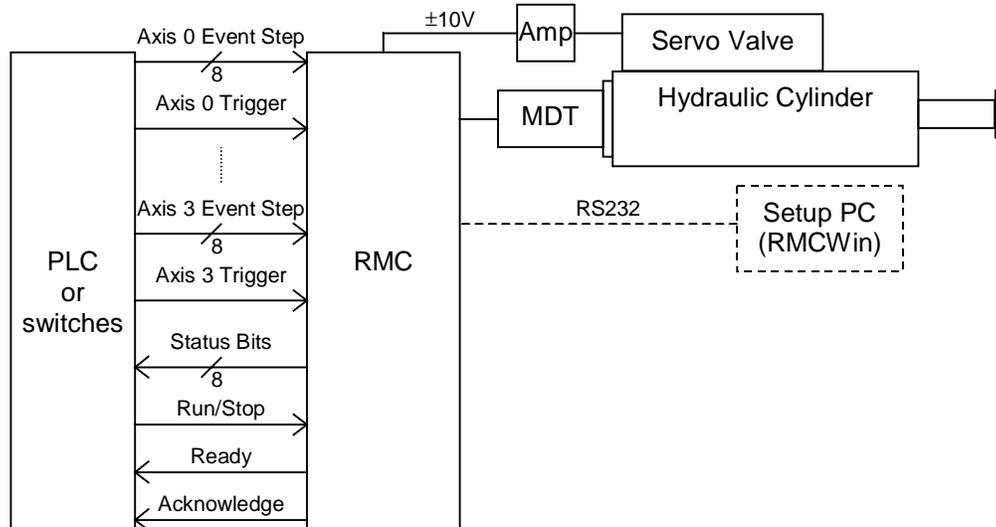
This document discusses only the connections between the Programmable Controller and the RMC. For details on the transducer and drive wiring, look up **Wiring Notes** in the RMCWin index.
