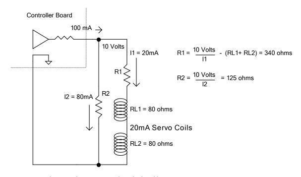
Resistor network power dissipation can be calculated by:
