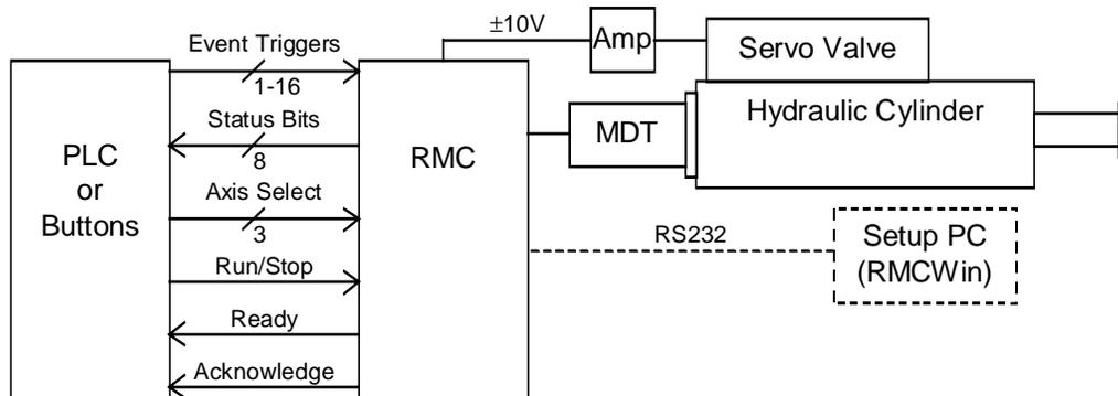
This document discusses only the connections between the Programmable Controller and the RMC. For details on the transducer and drive wiring, look up **Wiring Notes** in the RMCWin index.
