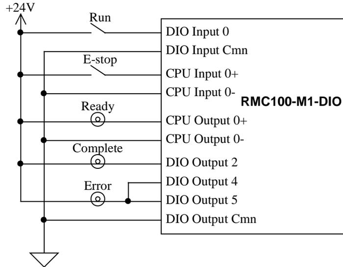
Simply by wiring the system, many of the controls are already handled:
